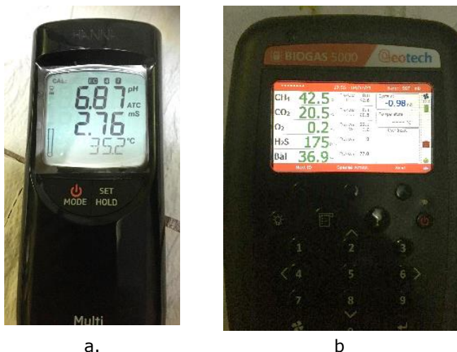
Figure 7. Portable equipment used for periodic measurements of gas composition, electrical conductivity, and pH: a) biogas analyzer and b) portable meter[1].
